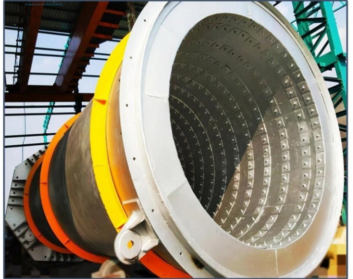
Bypass Stack With Super Wool Insulation
