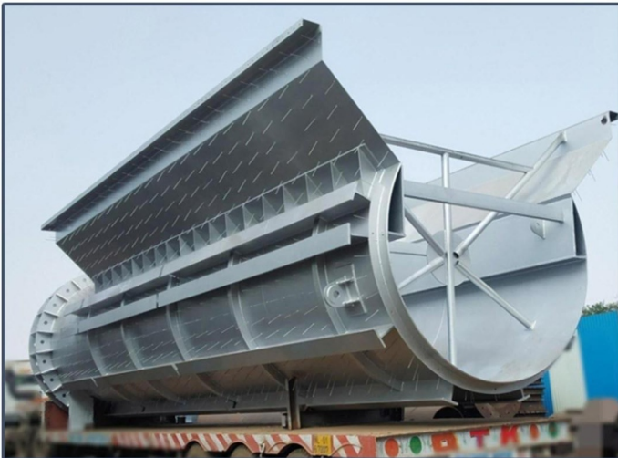
Bypass Stack With Duct
